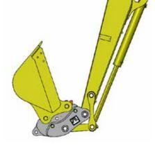
Rotate attachment to transport position.
