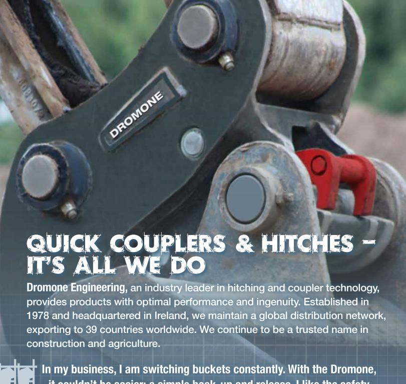
In my business, I am switching buckets constantly. With the Dromone, it couldn't be easier: a simple hook-up and release. I like the safety of this coupler – especially the snap-on front lock. When it snaps on, it's locked. All I need now is the next one to be delivered.
