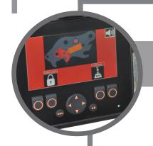
In cab controls notify operator of failed connection.
